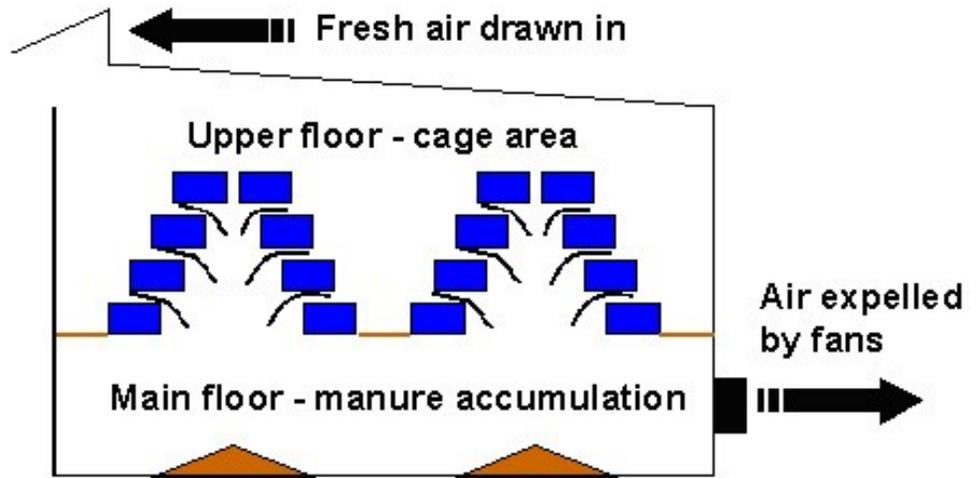
**Figure 1.** Schematic of a high-rise layer structure. Fans in the wall of the structure draw air out under negative pressure (suction). This pathway of air flow serves to vent ammonia and other gasses out of the structure, minimizing exposure of poultry.
