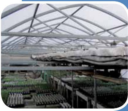
Scott Sanford developed on-line tools for educators to deliver programming on energy management and conservation for greenhouse production, such as these thermal/shade curtain systems. Photo by Scott Sanford.
